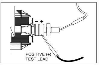
Figure 9. Testing Rotor Insulation (12-20kW)
